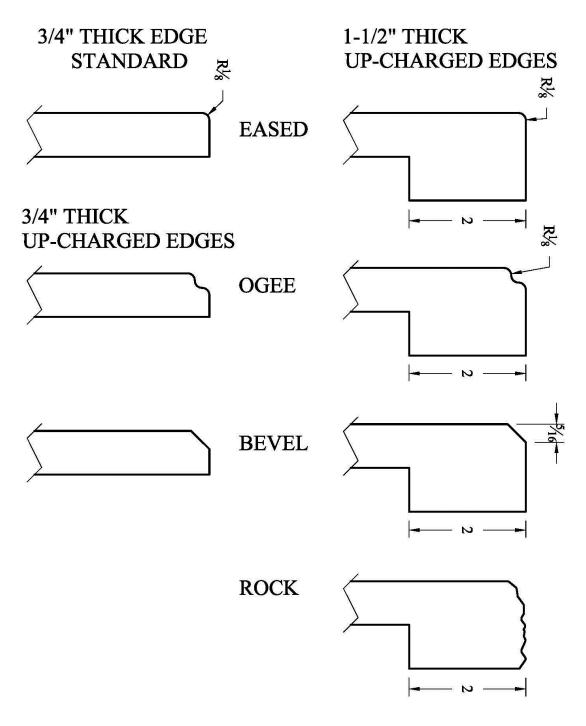
NOTE: 1-1/2" THICK BUILT UP EDGES ARE DESIGNED TO SIT ON TOP OF CABINET
